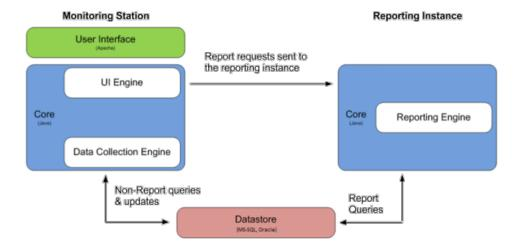
In this deployment configuration, the Monitoring Station is still the main point of interaction for all up.time users; no one can log in to the reporting instance Web interface. When the Monitoring Station receives a report generation request or is scheduled to generate one, it seamlessly offloads the request to the reporting instance. Generated reports are stored on the reporting instance, which by default are the following:
