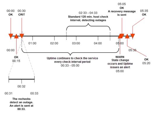
All service monitors have a common set of Monitor Alert Settings that configure aspects of the alert flow.
