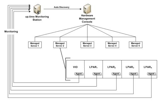
In order to monitor the managed servers and their LPARs, up.time must communicate with the HMC.
