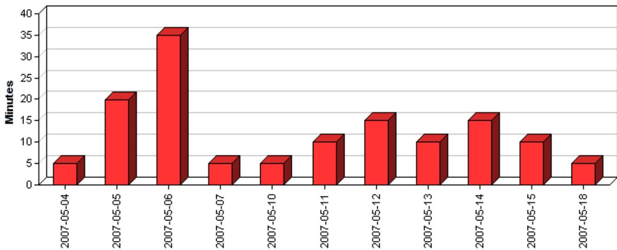
In this example, the system is consistently over the run queue threshold that was specified when the report was defined. Based on this information, you can generate a CPU performance graph (see [See Monitoring CPU Performance](#) for more information) to get a better idea of why the system is exceeding the CPU run queue threshold.
