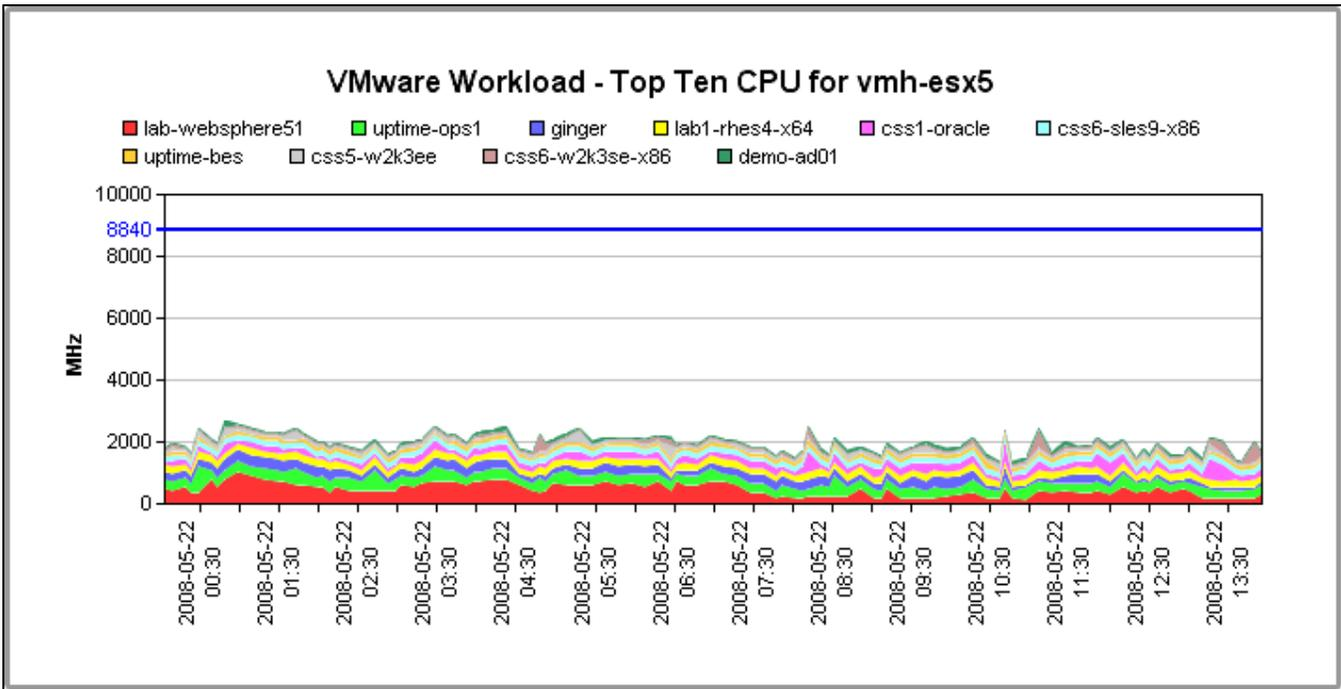
This graph indicates that, on average, the 10 most CPU-intensive instances use only 20% of the server's CPU capacity. The CPU on the server can handle up to three to four times its current load.
